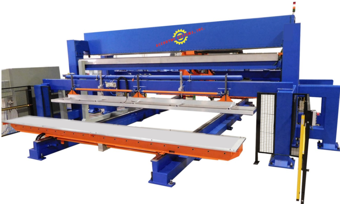
Figure 5: Stringer Former and Trim Cell
