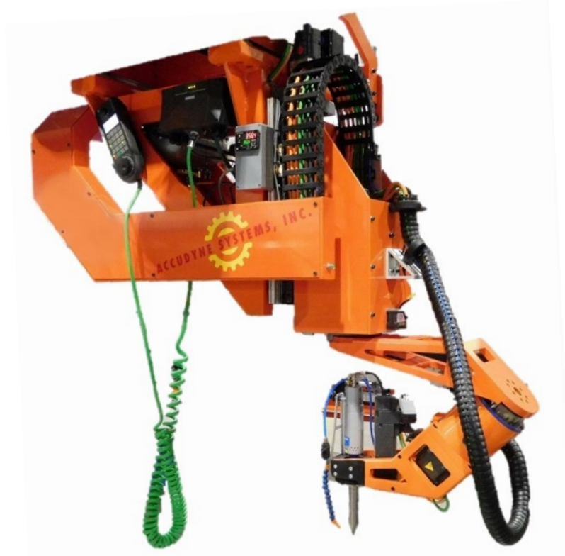
Figure 8: Stringer Former and Trim Cell Ultrasonic Trim Head
