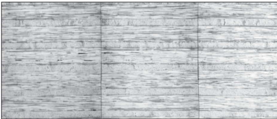
Figure 9. Quality was high with at 0.9% void volume fraction, no hoop waviness, and little axial waviness. The ultrasonic C-scan was uniform.
