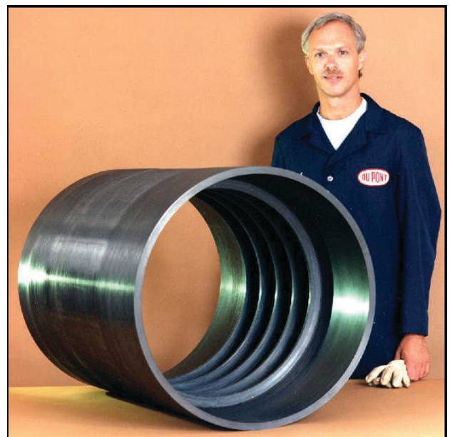
Figure 1. The APC-2/AS-4 ring-stiffened cylinder had a [90^\circ_{2.27}/0^\circ]_n laminate stacking sequence and five integral 90^\circ ring stiffeners.
