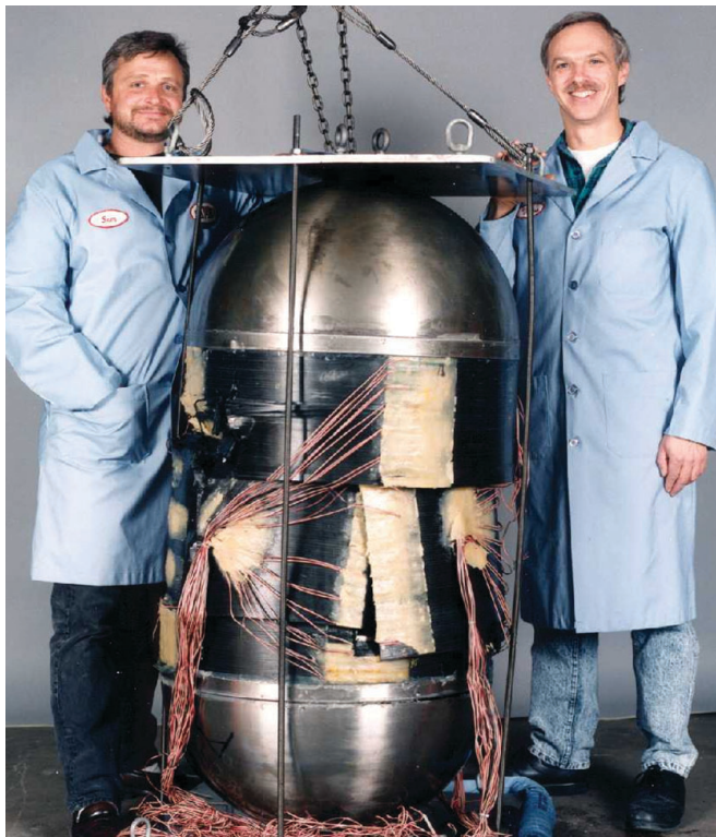
Figure 12. In the test, the cylinder failed at 37.9 MPa (5500 psi), within 3% of prediction.
